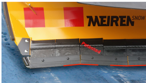
Patented, road surface copying blade holders clean the road surface and smoothly overcome obstacles
